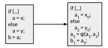
• Solution: introduce a  $\varphi$ -function ("phi function")
