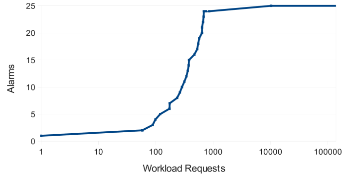
Fig. 6. Alarms raised by N-Prog applied to a webserver with no test cases against an indicative workload of 138,266 requests (note log scale). Each alarm corresponds to a test case (input and oracle) discovered. The last alarm is raised at request 10,212.
